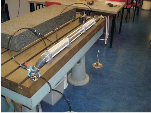
Figure 3.7: Second test setup for pneumatic cylinders. (Festo DNG-40-200)
