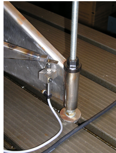
Figure 3.10: The end of the measuring arm and the probe, fixed on the arm, attached to the fixed pulley halve and the table
