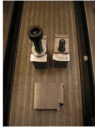
Figure 3.4: On the left side is the clamp used to fix the plate on the moving pulley halve, on the right side, the one for the fixed pulley halve
