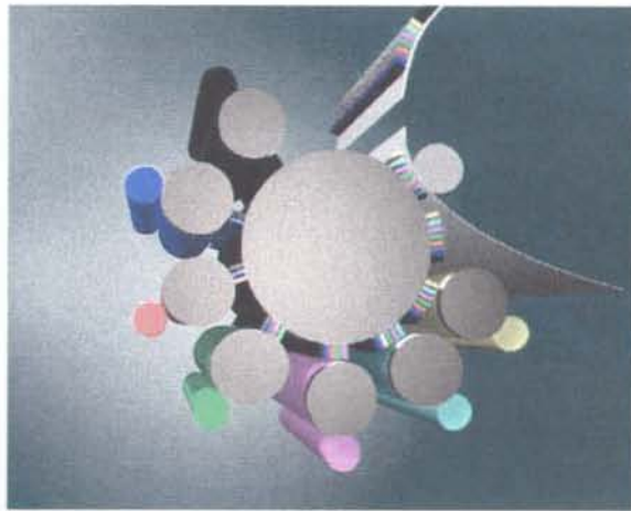
Figure 1.1: The DIP-setup with 7 DIP-units, each developing a monochrome color image onto the intermediate before it is transferred to the paper.
