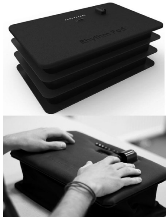
Fig. 5. Example Paced Breathing: Rhythm Pad 3D render (top) and prototype (bottom) including feedback on Heart Rate Variability – TU/e student project by Sergej Lojko
