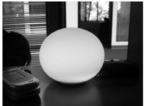
Fig. 1. Ambient Orb by Ambient devices. The colour of this lamp changes to inform about the weather conditions. The change in colour can also show other kinds of digital data, according to user's preferences.
