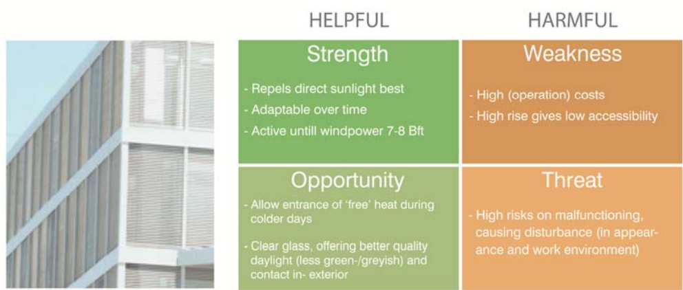
Figure 8. External sunshading principle
