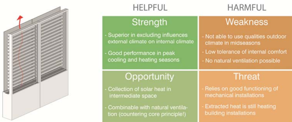
Figure 5. Characteristics climate façade
