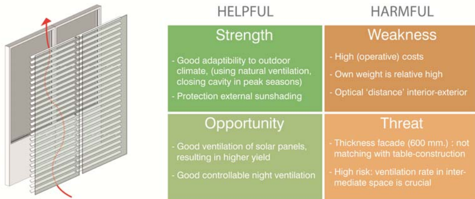
Figure 6. Characteristics double skin façade
