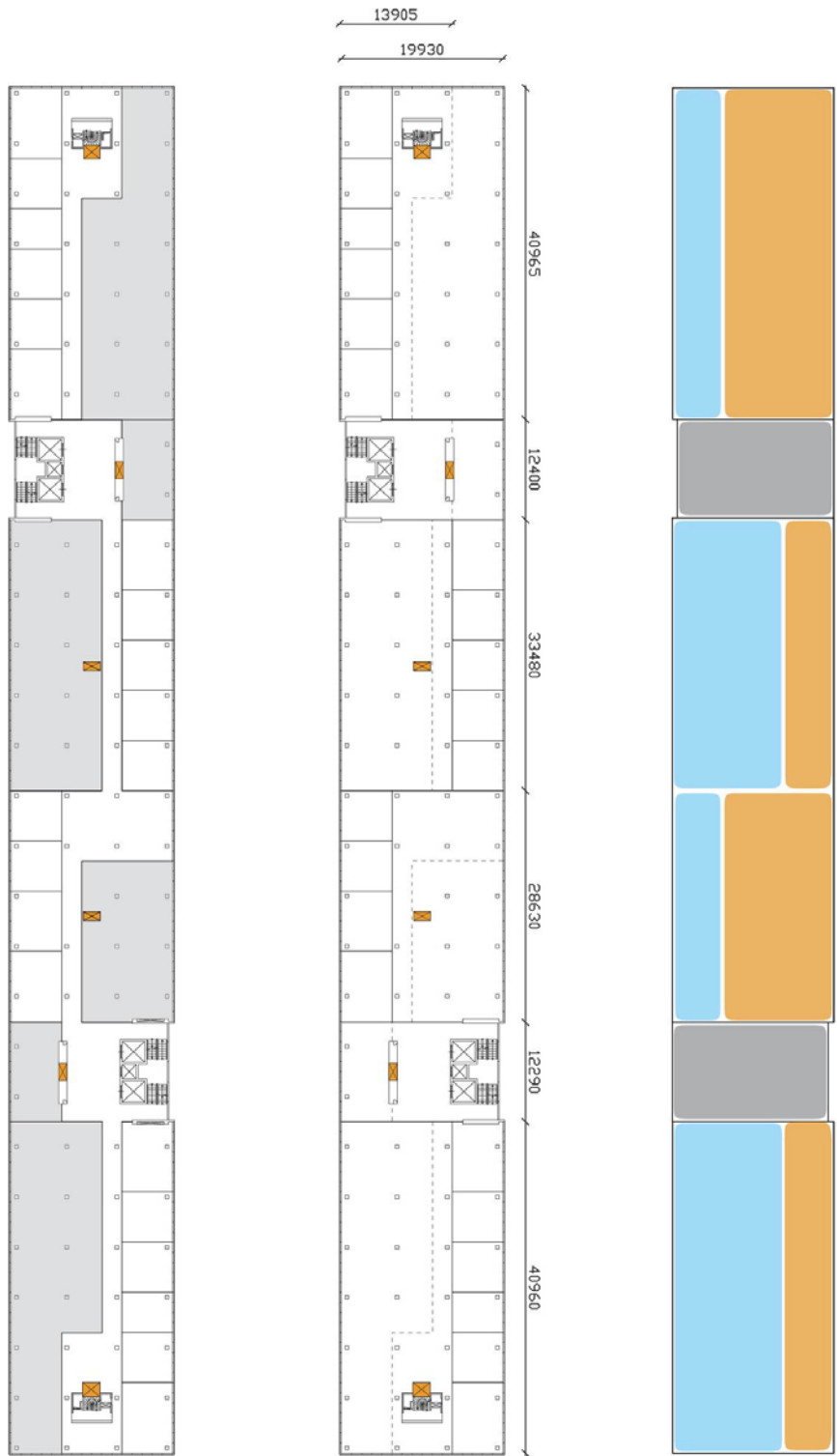
Figure 30. Organisation principle, floor plan. (left: flexible floor; middle: structural floor, right: zoning)
