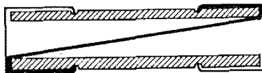
Fig. 1 Design of a miniature fuse using a plastic body and no sand filler.
