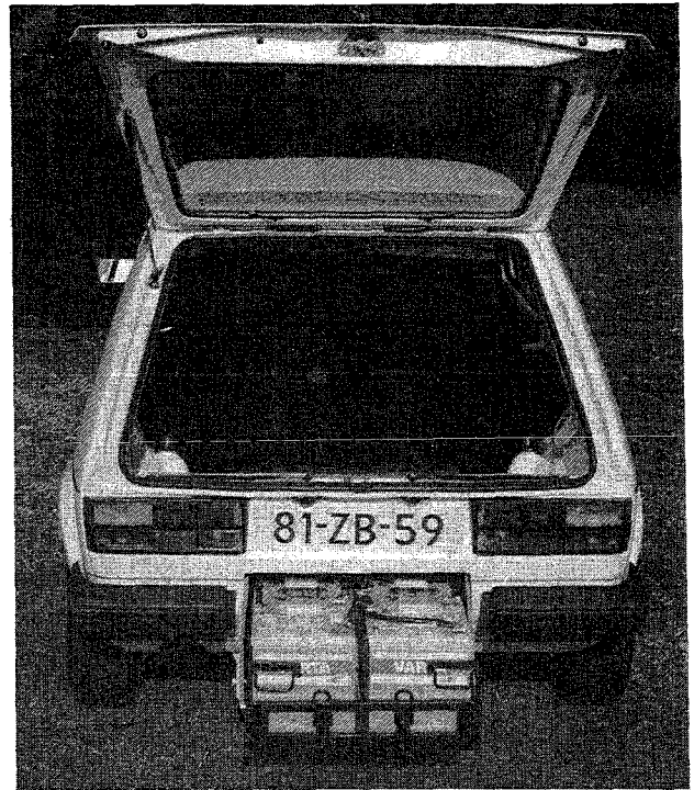
Fig. 2 Interior of the modified Golf, showing the battery case construction
