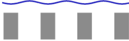
Figure 3.1. Schematic of flame curvature above the burner plate.
