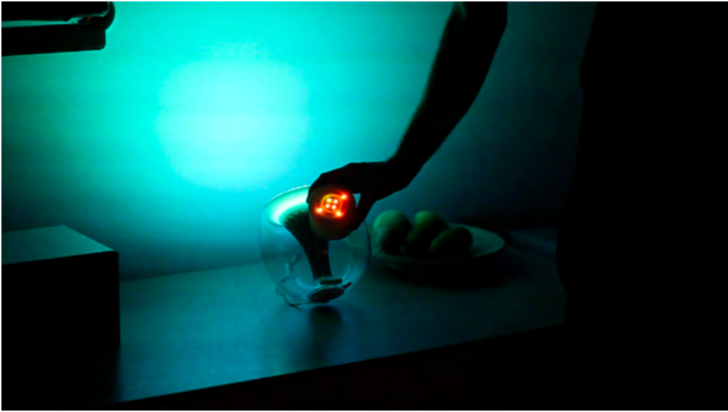
Figure 4.5: Image showing the Connector scanning a coloured lighting lamp.
