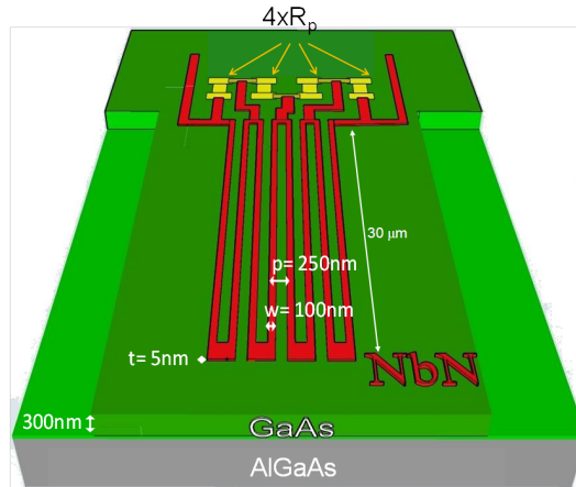
Figure 6.1 – Schematic of a waveguide photon-number-resolving detector (WPNRD) consisting of four wires in series with a resistance ( R_p ) in parallel to each wire (contact pads are not shown).
