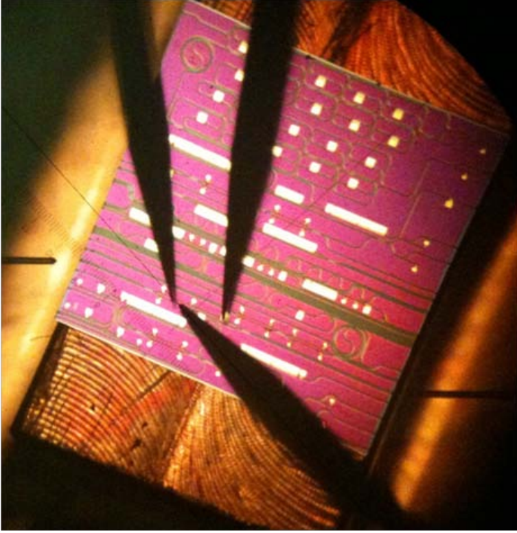
Figure 5.13: BOTDR PIC bonded with epoxy on a copper sub-mount for the measurements.
