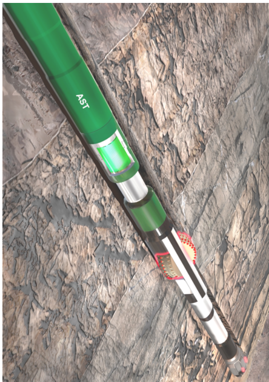
Figure 7.1: Impression of the anti stick-slip tool (AST) placed in the drill-string near the bit [112].
