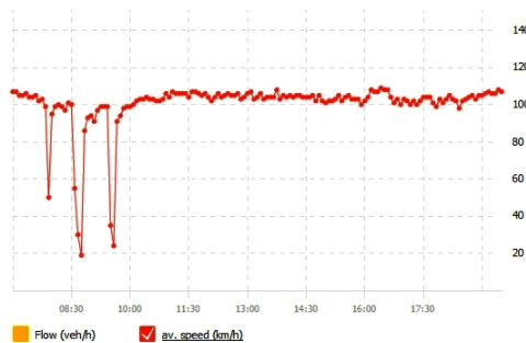
Figure 1.1 Average speed profile at highway A12 on the 19 th September 2013 (Regio Delft Project 2013)
