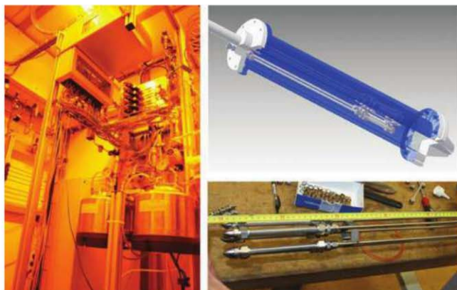
Fig. 1 Test-rig and multi-tube membrane reactor available at TU/e (membrane bundle visible in the right corner)
