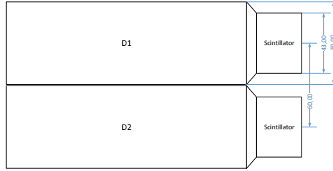
Figure 4.5: How the two cylindrical \text{LaBr}_3 scintillation detectors are placed next to each other. The detectors register an X-ray signal simultaneously during some discharges. This proves that the photon flux is high enough to cause a multiphoton registration at one detector.
