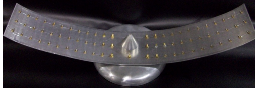
Figure 2.6: Our alternative grounded electrode of 55 by 10 cm with 75 sharp points to generate upward negative streamers.
