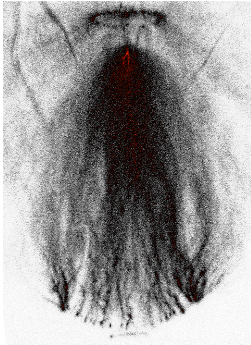
Figure 2.7: Connection between positive downward and negative upward streamers initiated from the sharp belt. Exposure time is 300 ns; the gap length is 1 meter.
