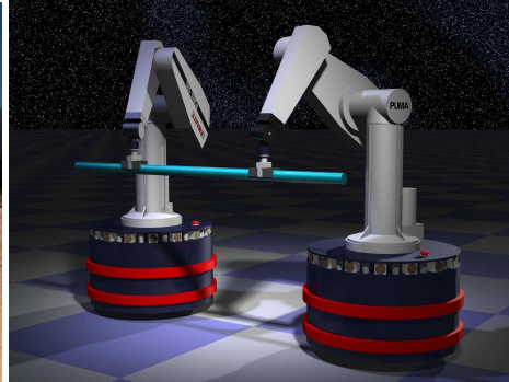
(b) Model of two Stanford Assistant Mobile Manipulators handling a large object [151].
