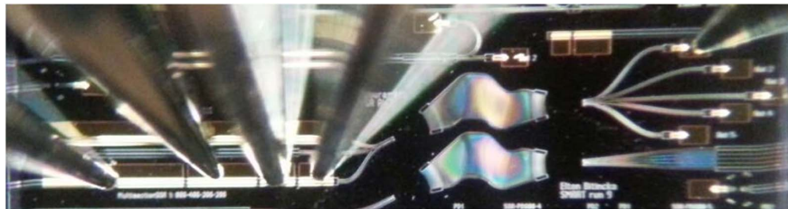
FIGURE 6.19: Microscope photograph of the on-wafer gain measurement test module while measuring. The measurement is realized through electrical signals only.
