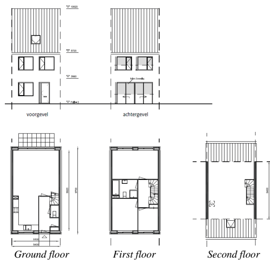
Figure-4 A typical Dutch corner terraced house (RVO, 2013).
