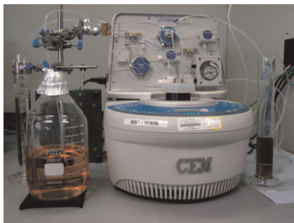
Figure 8. Photograph of the stop-flow Voyager [92] (reprinted with permission from [92]). Copyright (2008) American Chemical Society.
