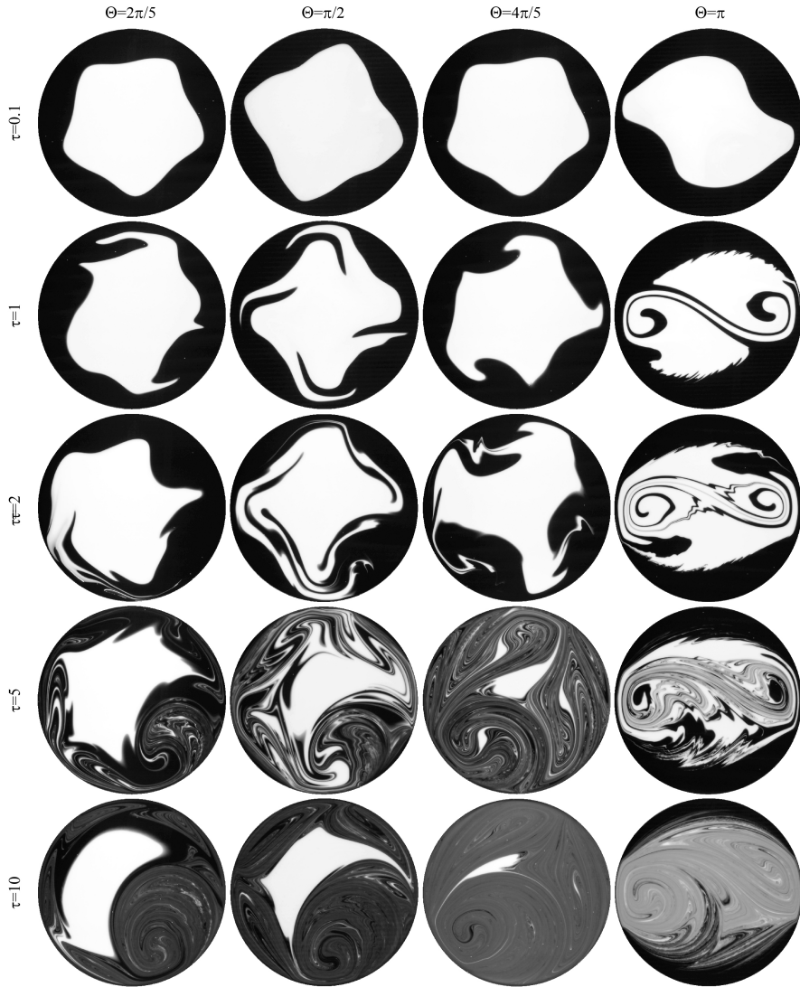
Figure 5.10: Experimental scalar patterns for the offset angles of \Theta = 2\pi/5, \pi/2, 4\pi/5, 2\pi and aperture activation time values of \tau = 0.1, 1, 2, 5 and 10 visualized after 20\tau .
