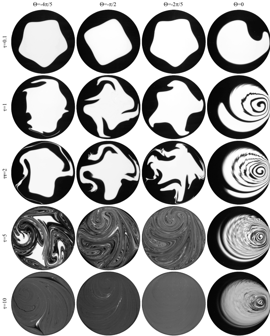
Figure 5.9: Experimental scalar patterns for the offset angles of \Theta = -4\pi/5, -\pi/2, -2\pi/5, 0 and aperture activation time values of \tau = 0.1, 1, 2, 5 and 10 visualized after 20\tau .
