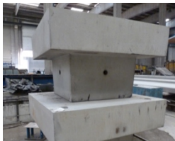
Figure 4. Precast isolated footings
