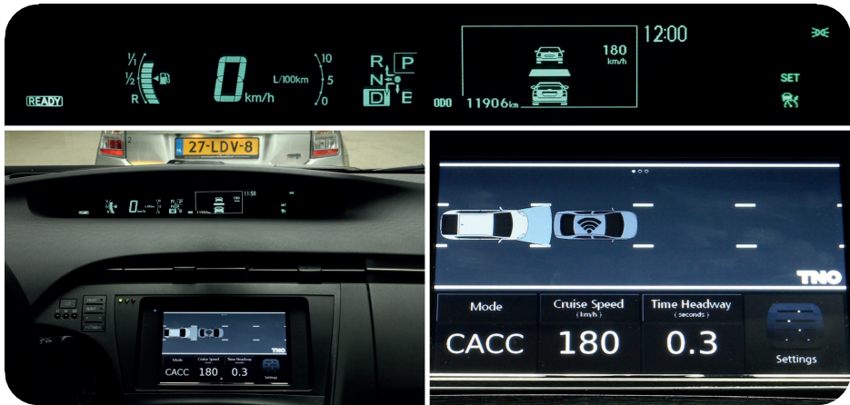
Figure 5.7: Human-machine interfaces in the dashboard: overview (bottom left), close-up of the CACC display (bottom right), and close-up of the native vehicle display (top).
