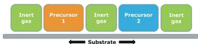
FIG. 10. (Color online) Scheme for spatial ALD where the precursors flow simultaneously and precursors are separated by inert gas zones.
