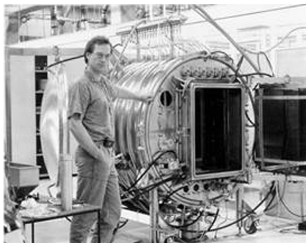
Fig. 3. Jarmo Skarp in 1985 standing next to a Planar P1000 reactor used in TFEL display production.
