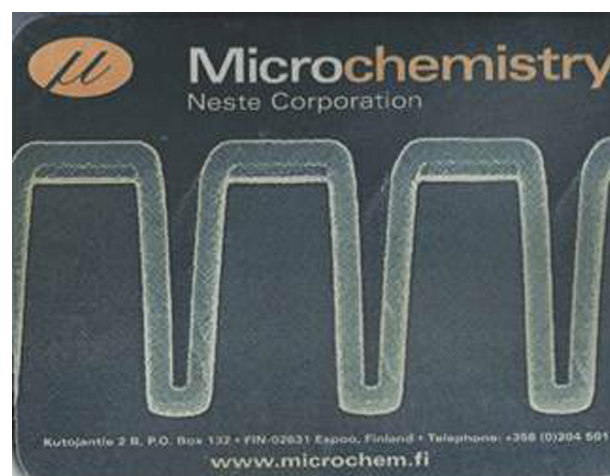
Fig. 5. (Color online) Photograph of promotional mousepad distributed by Microchemistry, Ltd. showing the excellent conformality of \text{Al}_2\text{O}_3 ALD on a trenched silicon wafer. Original photo was published in M. Ritala, M. Leskelä, J.-P. Dekker, C. Mutsaers, P. J. Soininen, and J. Skarp, "Perfectly conformal TiN and \text{Al}_2\text{O}_3 films deposited by atomic layer deposition," Chem. Vapor Dep. 5(1), 7-9 (1999).
