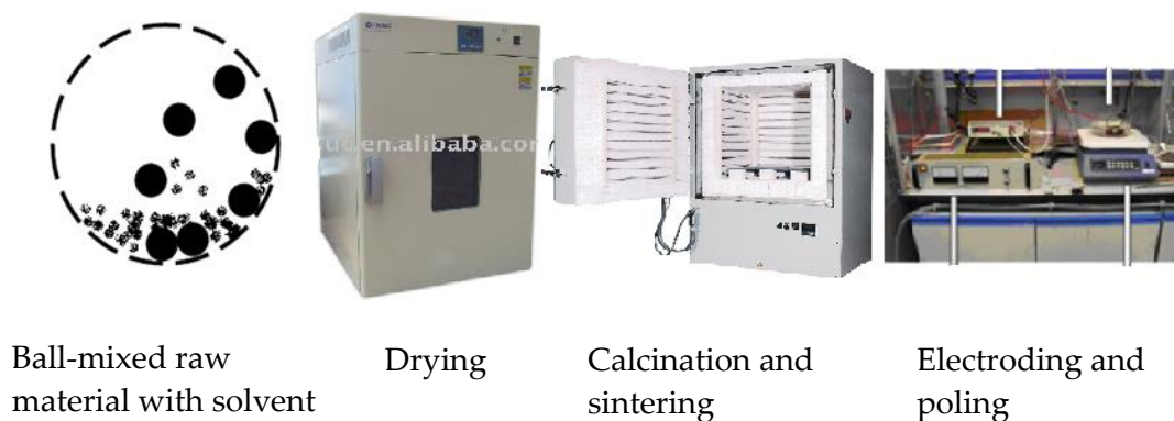
Figure 8. Manufacturing process of PZT.
