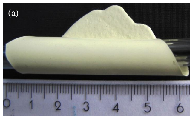
Figure 1 (a). Photograph showing the flexibility of a 40 vol. % PZT-PDMS composite film (thickness \sim 280 \mu\text{m} ).
