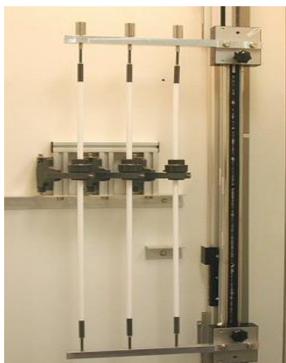
Figure 8.2: Experimental set-up used to impregnate the membrane with the IL [emim][FAP]
