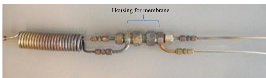
Figure 8.5: Module with 10 cm housing for tubular membranes.
