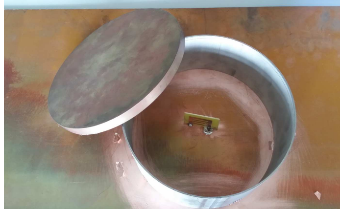
Figure 4.20. Radiation efficiency measurement setup using a cylindrical cap.
