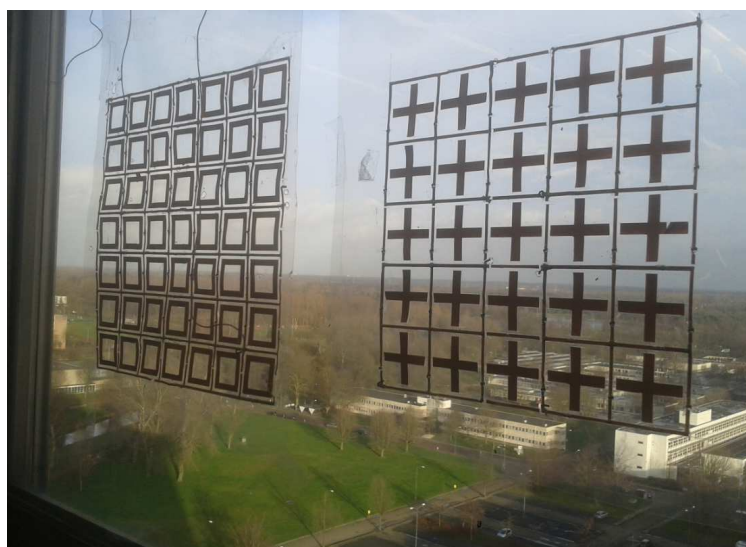
Figure 7.1. RF power harvesting glass using frequency selective surfaces.
