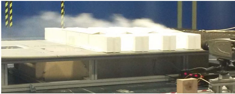
Fig. 5: Smoke visualization over an array of blocks to simulate an urban canyon.
