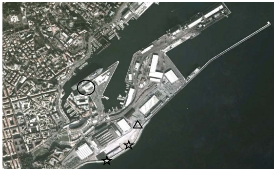
Fig. 1: Savona Harbour with the location of the solar photovoltaic system (circle), the wind turbines (stars), the sonic anemometer (triangle)
