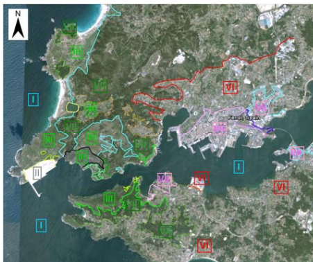
Fig. 6: Subdivision of local terrain into patches based on roughness classification and corresponding roughness categories and parameters z_0 , k_s and C_s .
