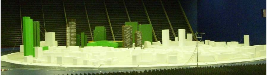
Fig. 3: Bosco Verticale buildings placed in the wind tunnel around the surrounding
