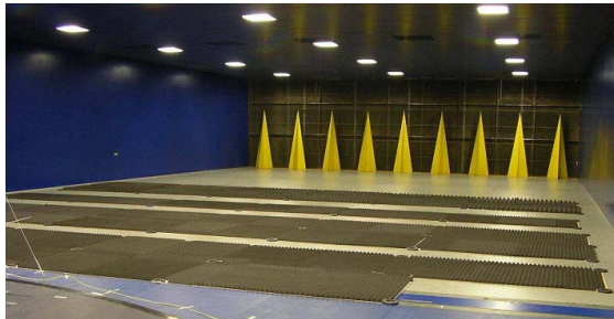
a) Polimi wind tunnel with spires and floor roughness
