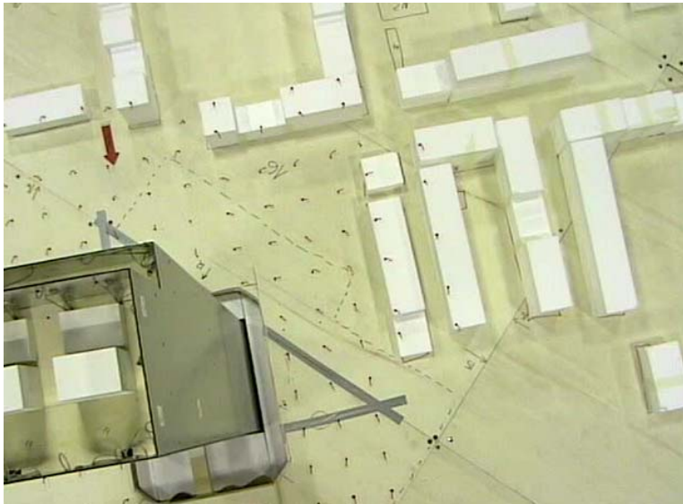
Fig. 7: Flow visualization in urban area with sewing threads.
