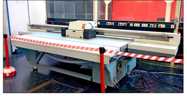
Fig. 3. Océ Arizona 550GT flatbed printer experimental setup. The printer is normally used to print on rigid media with applications in interior decoration, product decoration, signage, and art.
