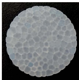
Figure 6.3: Final disk-shaped sample, 32 mm in diameter with near-virgin melting and crystallization kinetics.
