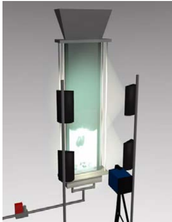
Pseudo 2D PIV setup with visual high speed camera (2016 x 2016 px @1600 Hz)
