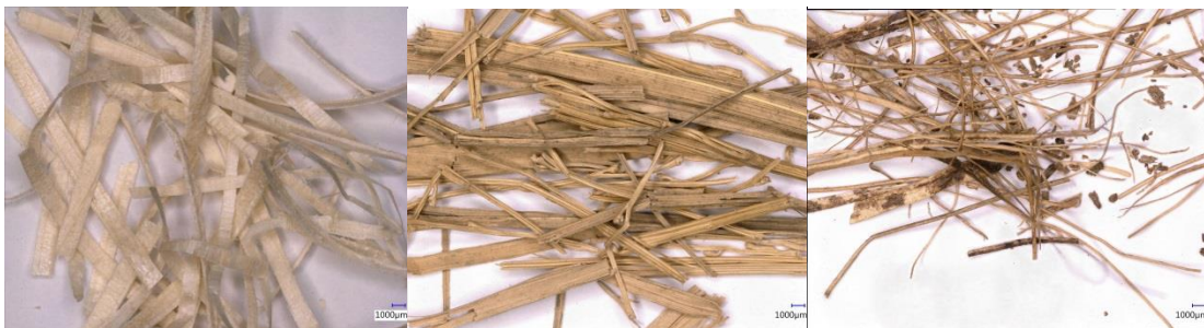
Fig. 2: Organic fibres – from left to right spruce wood, rice fibres and coconut fibres
