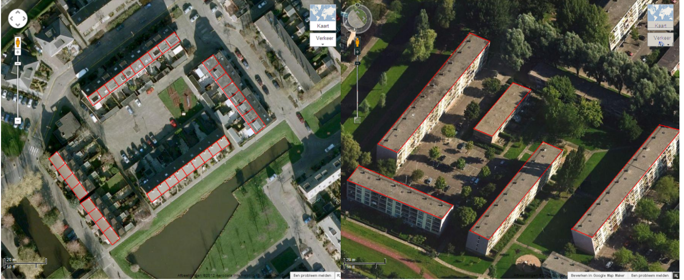
Fig. 1. Satellite images to determine available roof area for PV (courtesy of Google Maps).
