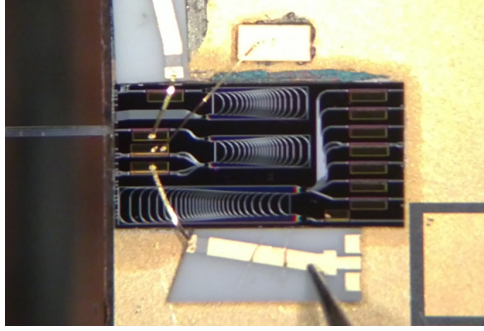
Fig. 3. Wire-bonded 4-channel AWGL on measurement setup. The device was placed in a 2 mm \times 4 mm cell.
