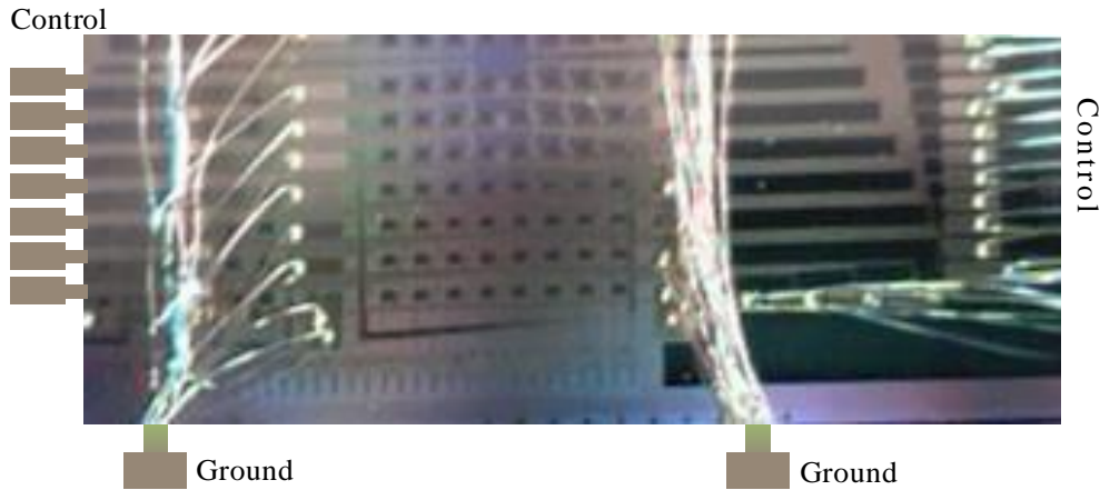
Fig. 1. Photograph of assembled circuit. Wire bonds leading to the left and right of the image are control lines. Wire bonds leading to the bottom edge are the common ground lines.
