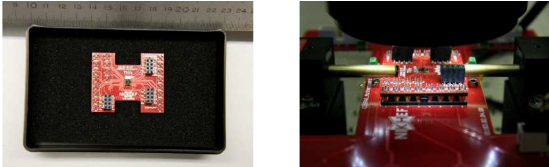
Fig. 3: (L to R) ASPIC glued and bonded on the sub-mount measuring 5×5 cm 2 . Sub-mount mounted on the motherboard for measurements.
