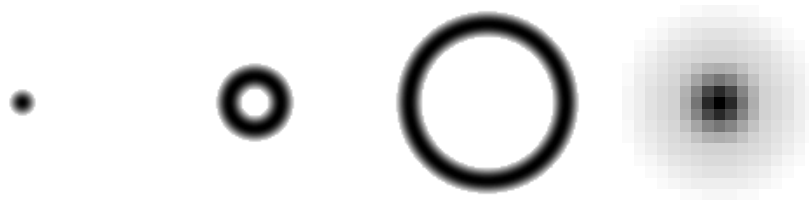
Figure 4.3: Basis functions of the parametric model in 2D. The first three plots on the left show 3 basis functions created using Eq.4.4. The rightmost plot shows the constructed PSF. The basis function are circular symmetric in the radial (XY) plane to ensure that the estimated PSF is also circular symmetric.
