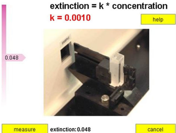
Fig. 4 Extinction formula. Only the formula is given, with no calibration line, in order to stimulate students to use the formula
