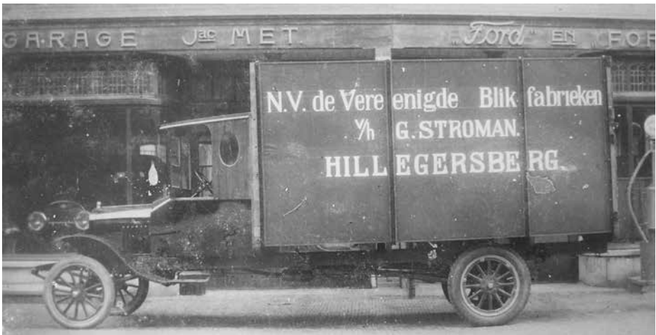
Figure 3.4 Lengthening a Model-T Ford chassis to convert it into a transport vehicle, by Jacob Met in Alkmaar, 1910-1920.
