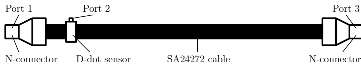
Figure 5.3: Drawing of the calibration setup. The SA24272 cable is fitted with N-connectors so that it can be connected to the vector network analyser.
