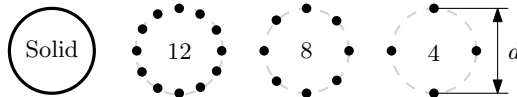
Figure 2.9: The four types of outer conductors used in the simulation results of Fig. 2.10 are: a solid cylinder and a cylindrical outer conductor made up of 12, 8 and 4 rods respectively.
