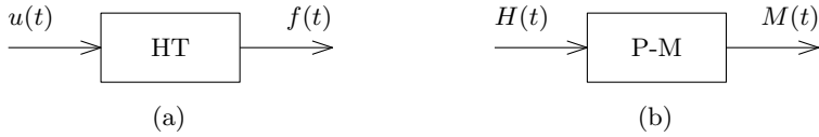
Fig. 5.1: Elementary model of hysteresis with, the hysteresis transducer (HT) (a), and the magnetic equivalent with the Preisach model (P-M) (b).
