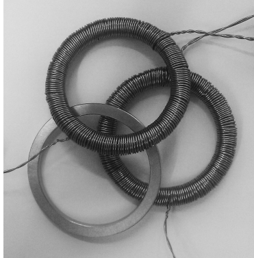
Fig. 3.6: Example of one solid toroid and two toroids with the applied primary and secondary coils.
