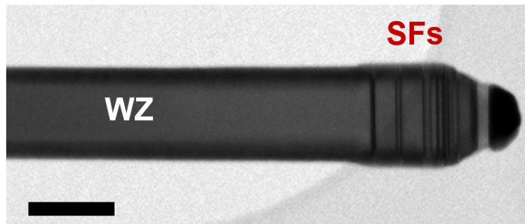
Figure 4.10: TEM image of a GaP/AlGaP core/shell nanowire showing the mixed phase AlGaP top axial segment. Scale bar: 100 nm.
