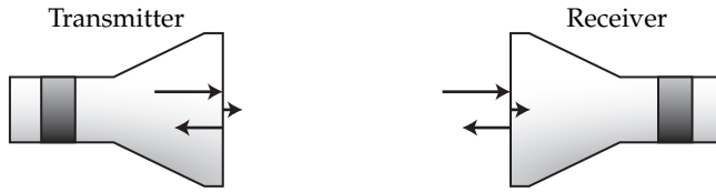
Figure 8.1 The transmission coefficient at the transducer-medium interface is very small for a poorly matched transducer. The wave that is reflected from the surface of the transmitter stays confined to the transmitter geometry and does not cause losses. The reflections on the receiver do cause losses due to absorption and diffraction.
