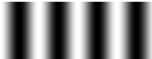
Figure 3.1 A longitudinal wave consists of successive areas of rarefaction and compression.
