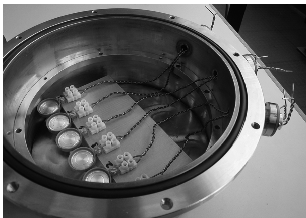
Figure 4.14 In vacuo impedance measurements were conducted using a small vacuum chamber. This allowed the simultaneous measurement of six transducers.
