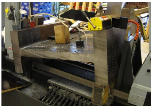
(c) Longitudinal saw-cuts for specimen A
