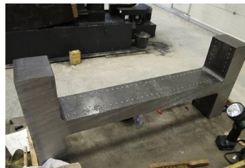
(b) Specimen E after transverse saw-cuts
