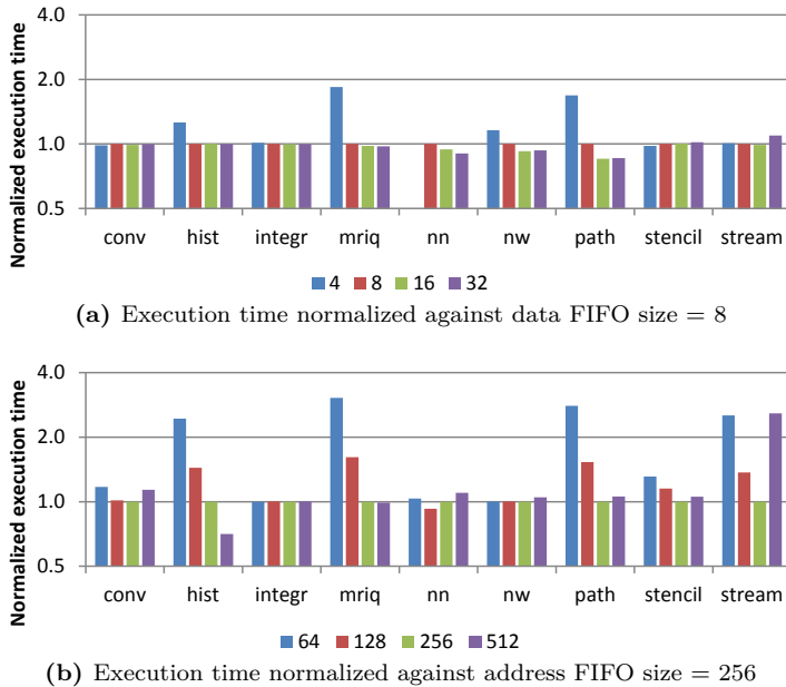
Figure 7.11: Normalized execution time for various FIFO sizes. The data FIFO sizes range from 4 to 32 (a) and the address FIFO sizes range from 64 to 512 (b).
