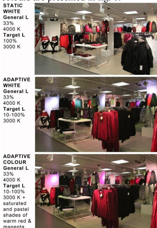
Fig. 1: The tested lighting schemes: Static, Adaptive White and Adaptive Colour.
