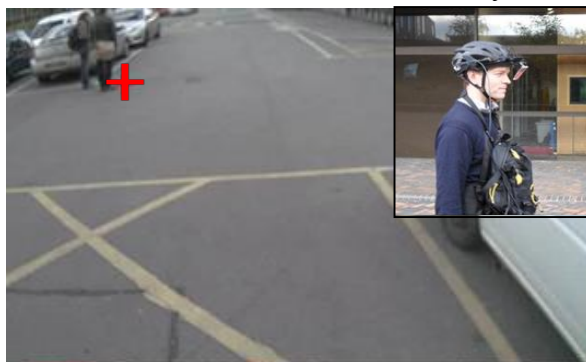
Fig. 1: SMI mobile eye-tracker system (inset) and screenshot from recorded video (main). Red cursor shows current point of gaze.
