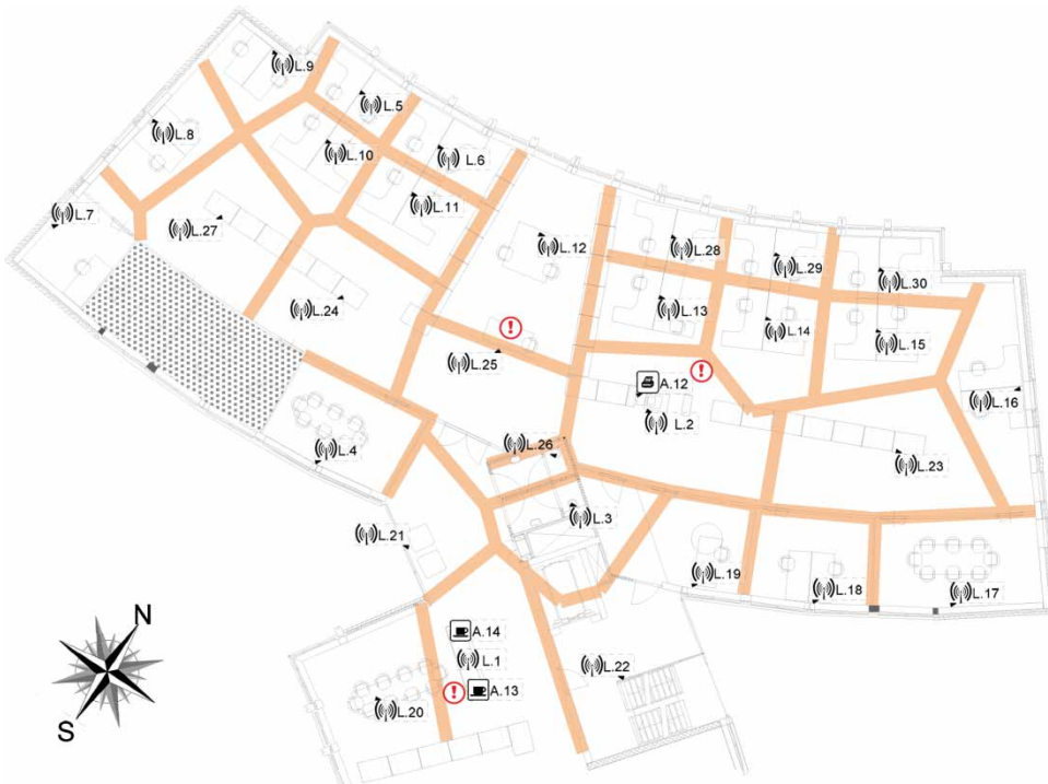
Figure 9. Positions of the static nodes creating a mesh of the zones for measuring the position of the building occupants on the floor. The transition region between the zones is marked by the broad light coloured line.
