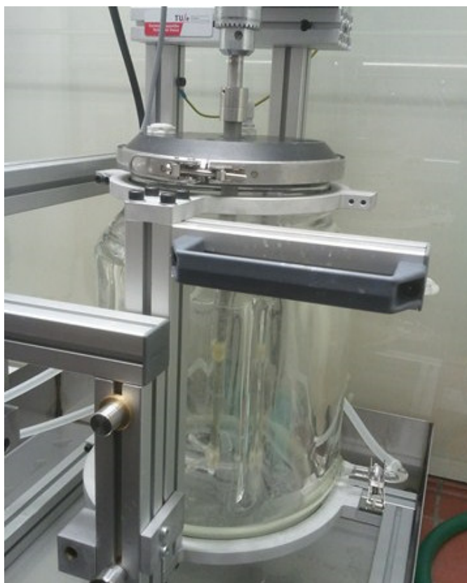
Figure 9.4. Reactor of 15 liters for the production of nano-silica.
