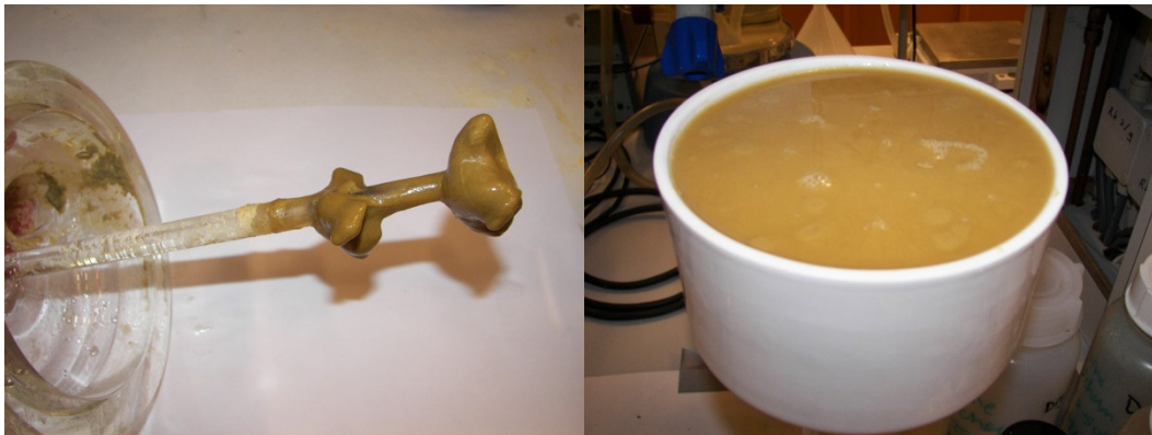
Figure 9.8. Thick mud produced when dissolving PROMGM-1 in sulfuric acid 3M.
