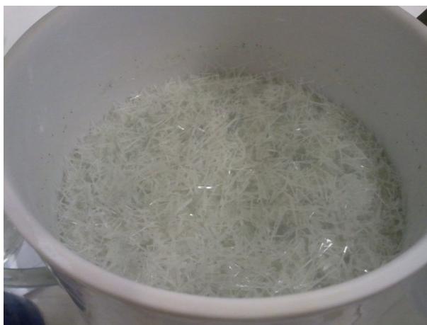
Figure 9.1 Formation of MgSO 4 needle crystals during filtration.
