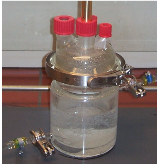
Figure 9.3. Reactor of 1 liter for the production of nano-silica.
