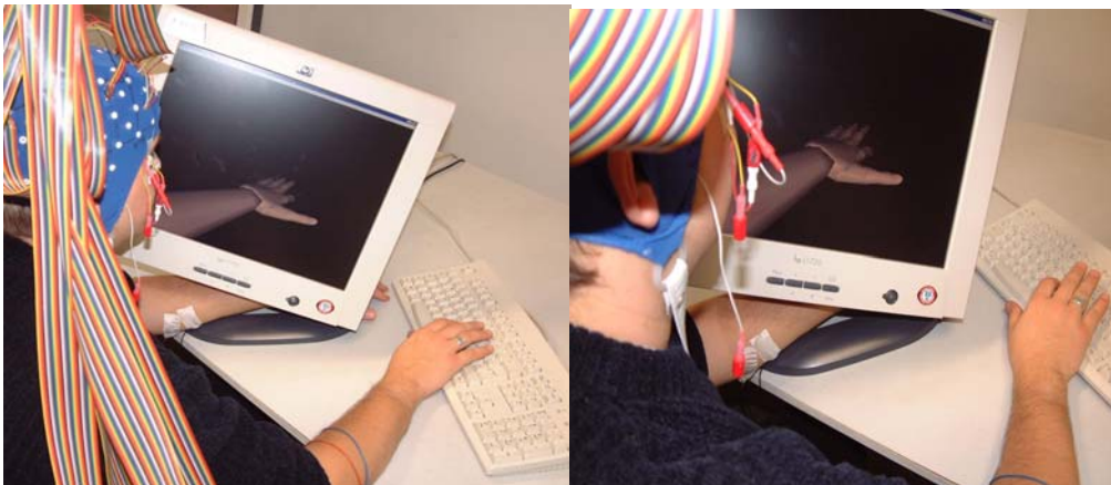
Figure 41: User and monitor position in experiments with the “Virtual Arm” feedback scenario. Monitor is placed and rotated such that the user’s imagination of observing the own arm while looking on the screen is maximized.
