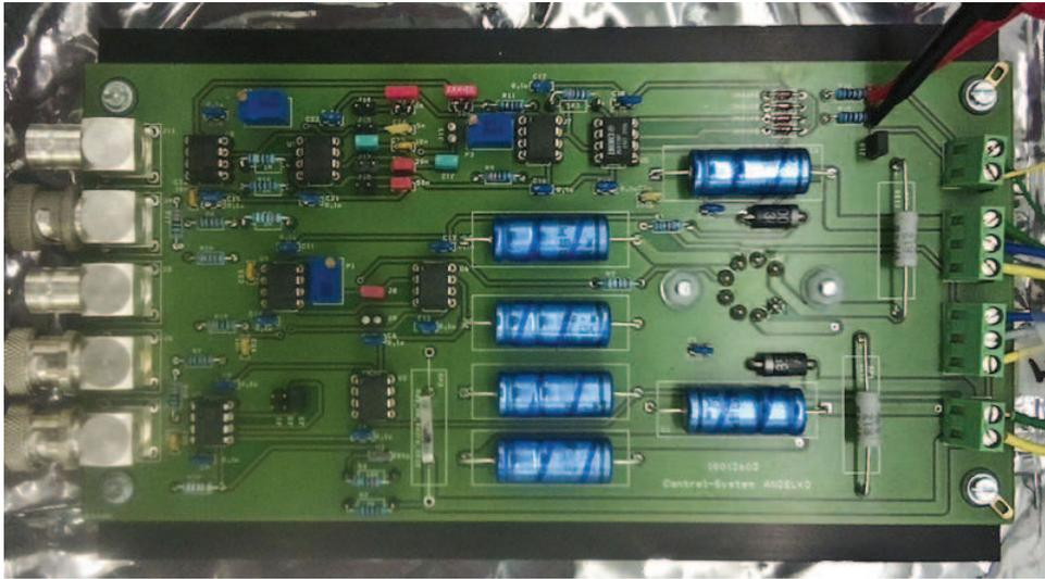
Figure 6.2: Image of the analog sensing coil voltage control circuitry (SCVCC)
