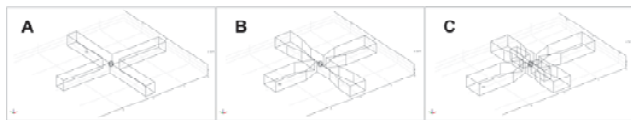
Figure 1: The cross slot designs used in the simulation. Design A: channel width and height are both 40 \mu\text{m} . Design B: the width is 50 \mu\text{m} , which is gradually narrowed to 15 \mu\text{m} in the x-direction and to 30 \mu\text{m} in the y-direction. Design C: channel width is 50 \mu\text{m} , narrowed to 15 \mu\text{m} in the x-direction, and the outlet channels in the y-direction contain obstructions.
