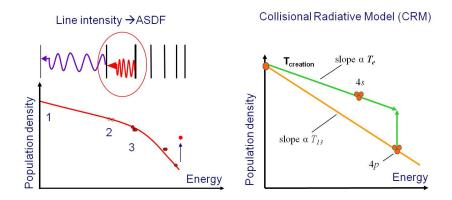
Fig. 1: Schematic of the Atomic States Distribution Function (ASDF) and the correction of the excitation temperature  $T_{13}$  into the creation temperature of the plasma via a CRM.
