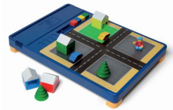
Figure 4.1. TagTiles console with an example application to train verbalizations of spatial relations. The playing pieces are localized and identified by the system. Visual effects are created with LED lights underneath the surface (top right square emits green light in this example).
